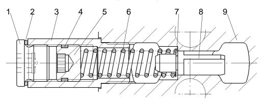
figure 6.1 - relief valves of pump types 101, 151 and 251
