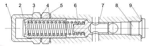
figure 6.2 - relief valves of pump types 51, 76, 351, 451 and 551
