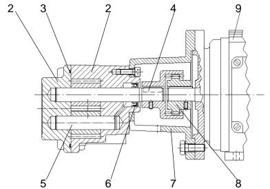
figure 4.8 - Pump with lip seal ring mounted to an electric motor
