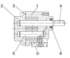
figure 4.5 – foot mounted pump with lip seal ring – e.g. to screw to a base plate
