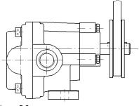
Driving pumps with a V-Belt Drive, Flat Belt Drive or multiple belt drive is only possible with pumps with an additional Ball Bearing for the shaft end (see section 4.2.4 - figure 4.14 and additional explanation). When calculating and choosing the belt drive, check the max. shaft end load of the used pump model.
